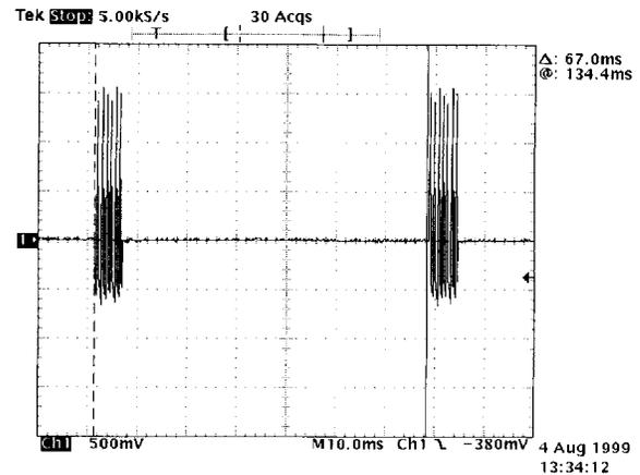
Fig. 3. Burst interval of Physio-Stim pulsed electromagnetic waveform as measured within the field coils.
